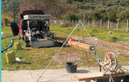
Colour video camera inspection in Greece. On the picture above the cable-disinfecting device can be seen.
